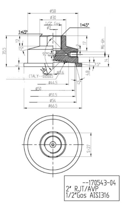
Note: Drawings are not to scale. All Dimensions are in mm.
