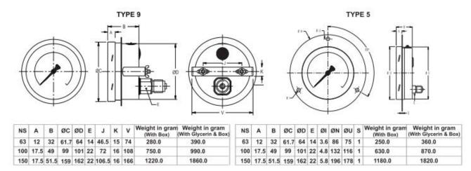
Note: Drawings are not to scale. All Dimensions are in mm.
